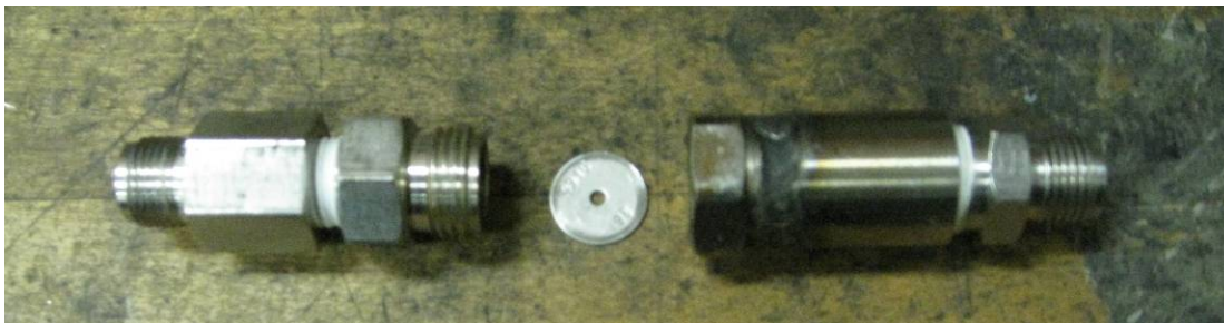
Figure 4 – Orifice plate flow restrictor.
